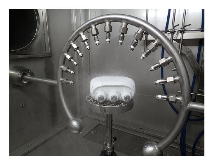
The IP protection class tests are type tests. Prototypes and samples are tested in the laboratory strictly in accordance with the specifications of the desired IP protection class. This involves testing the tightness against the ingress of particles and moisture.
