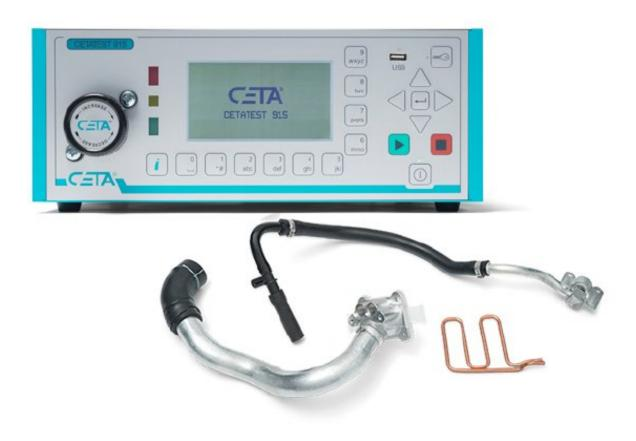
In addition to leak test devices, the CETA range of test devices also includes flow testers that use compressed air as the test medium. Thereby the principle of laminar flow measurement is used. Flow testing has a wide range of applications.
